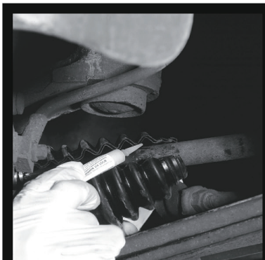
4. Start gluing at the small end in areas of 2 cm.
